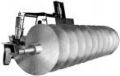
60 Inch Diameter Stainless Steel Steaming Vessel Screw Used in Handling Wood Chips.
