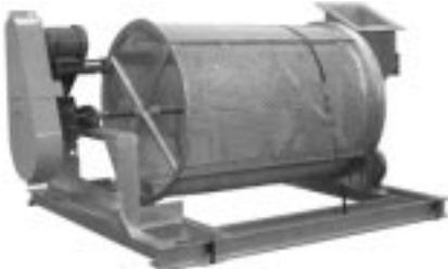
Rotary Screen Separator For Making Commercial Ice.
