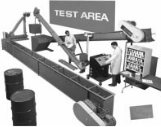
Test Facility. an Added Customer Service. This Area is Available to Check the Conveying Characteristics of Customers' Materials.
