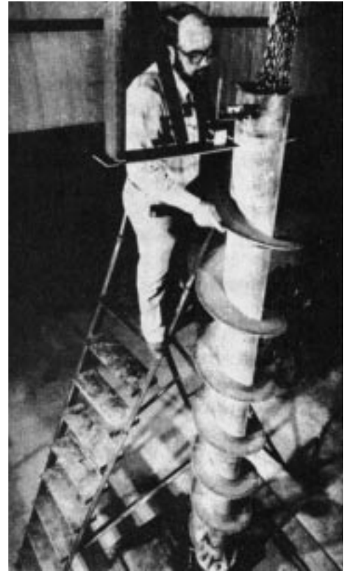
Inspecting total indicated runout of vertical screws.
