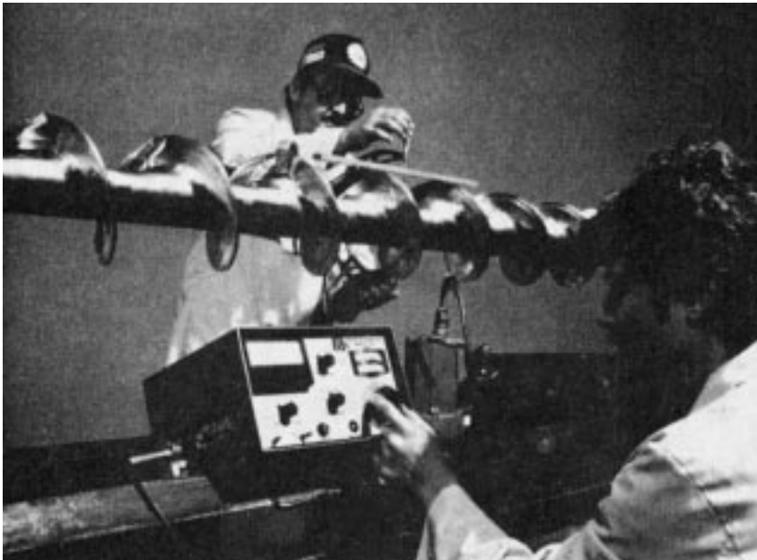
Dynamic/static balancing of screws takes place at one of Martin's manufacturing facilities.
